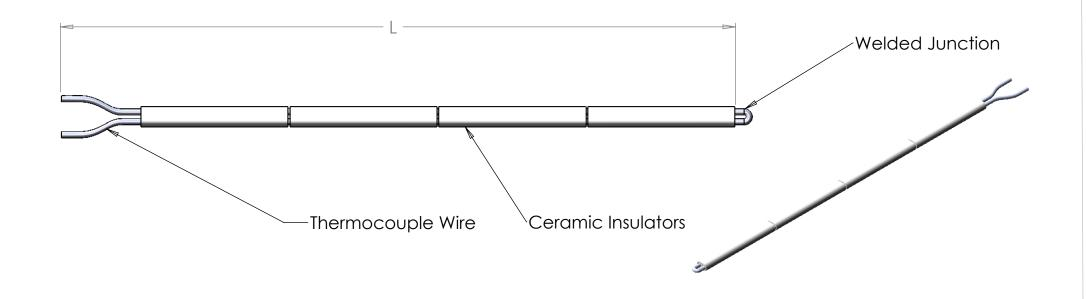
Note: 8 AWG = 3.2 mm 14 AWG = 1.6 mm
