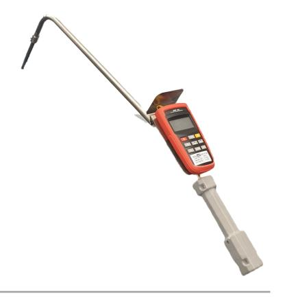
\*Removing one half of the grip exposes terminals for easy thermocouple replacement.
